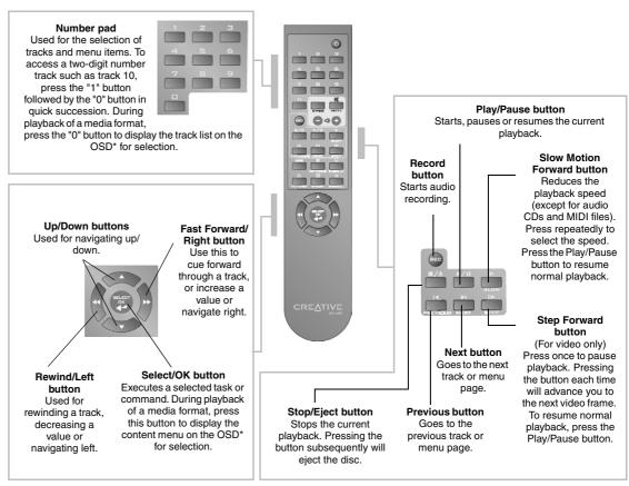
Figure 1-4: Navigation Buttons on the Remote Control.
